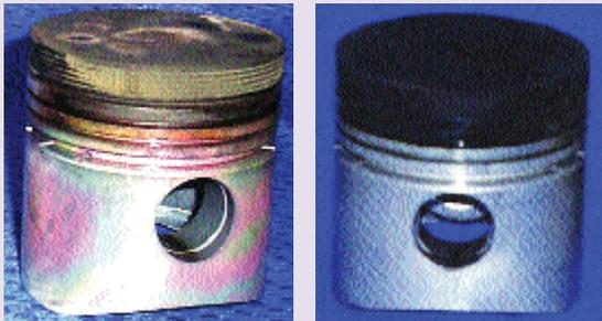
**Figure 1** A SilcoKlean™1000-treated piston (left) shows dramatically less coke buildup than an untreated diesel piston (right).
